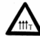
Lane Closed (Four Lane Road)
