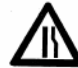
Right Lane Diverted
