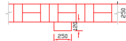
FIRST COURSE OF BOUNDARY WALL (BRICK)
