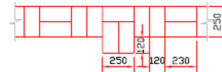
SECOND COURSE OF BOUNDARY WALL (BRICK)
