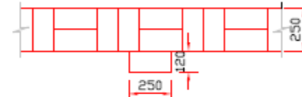
FIRST COURSE OF BOUNDARY WALL (BRICK)
