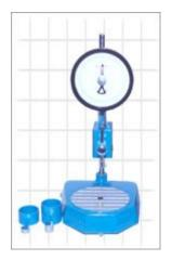
Penetration test for bitumen.
