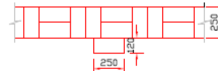
FIRST COURSE OF BOUNDARY WALL (BRICK)
