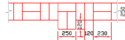
SECOND COURSE OF BOUNDARY WALL (BRICK)
