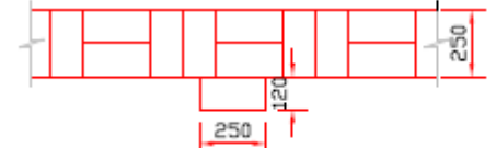
FIRST COURSE OF BOUNDARY WALL (BRICK)
